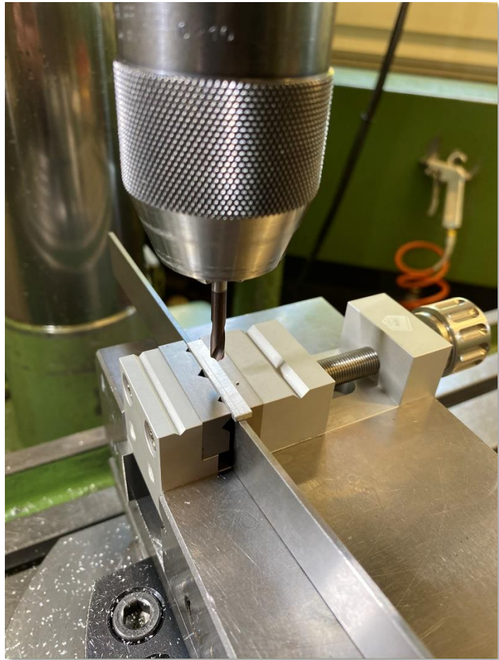
Abbildung 22 | Mounting Panel bohren
